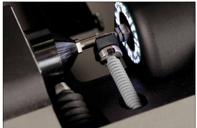
In the transfer mode, the 3D models of the rough stone and the optimized fancy shape are exported from the planning software of the rough planner to Eos Fancy. The operator then only has to align the rough scanner model to the actual rough in the Eos Fancy machine. The fancy shape coupled to the 3D-representation of the rough is centred automatically and bruted after a simulation of the bruting process.
