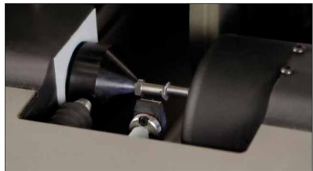
Photo 2: special designed pots to fix fancy shapes.
